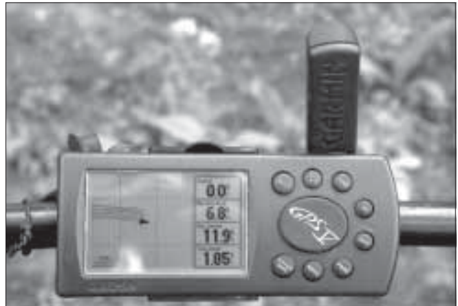
An ATV-mounted Global Positioning System (GPS) unit can be used to record the planting path.
